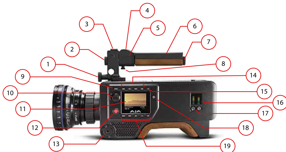
Figure 3. CION Operator Side
